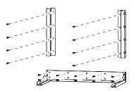
5 Slip connect the Shell to the upper brackets thru the eyelets.
