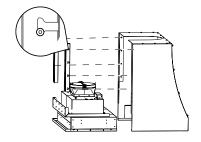
3 Secure the insert hood to the lower support.
