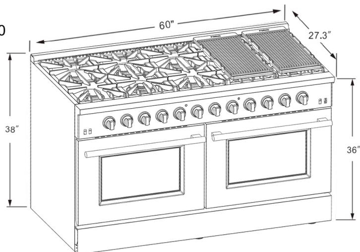
This range may be installed directly adjacent to existing countertop-height cabinets (36" or 91.5 cm from the floor). To achieve the best look, the cooktop should be level with the cabinet countertop. This can be accomplished by raising the unit using the adjustment spindles on the legs.
