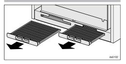
■ Remove the grease filters from the slots on the front of the housing.
