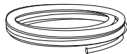
Hot water line with ferrule and compression nut - min 3/8" (9.5mm) copper tubing or flexible braided hose
