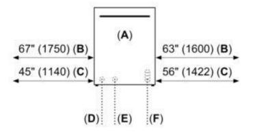
All connections are at the rear of the appliance. Extension for drain hose available as accessory.
