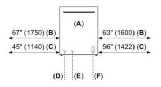
All connections are at the rear of the appliance. Extension for drain hose available as accessory. Junction Box for hard wired connection available as accessory.
