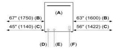
All connections are at the rear of the appliance. Extension for drain hose available as accessory. Junction Box for hard wired connection available as accessory.
