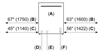
All connections are at the rear of the appliance. Extension for drain hose available as accessory. Junction Box for hard wired connection available as accessory.
