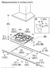
A: 51/16" (129 mm) required when installed with a built-in oven
