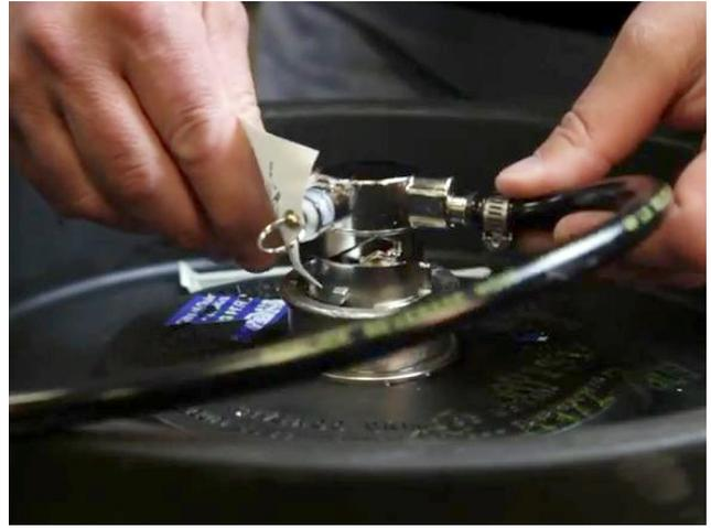
**CONNECTING THE REGULATOR TO THE CO2 CYLINDER**
