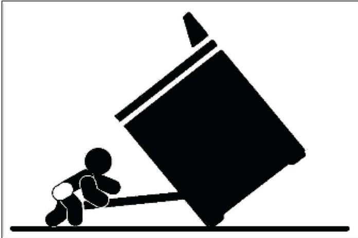
To reduce the risk of the appliance tipping, it must be secured and connected using the anti-tip device according to the installation instructions. Re-engage the anti-tip device if the range is moved.
