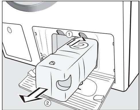
① To release the lock, press the yellow button above the cartridge.
