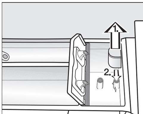
1. Remove the siphon from the
