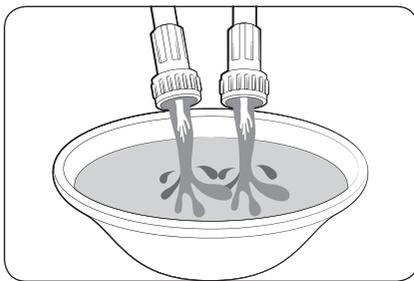
3. Put the other ends of the hoses into a bucket, and then open the water taps for 10 - 15 seconds to remove impurities. When done, close the taps.
