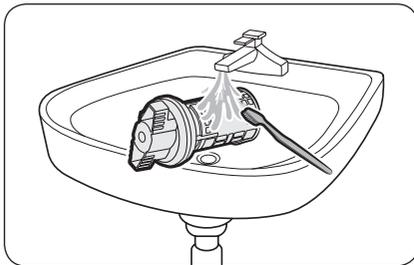
5. Clean the **drain filter** using a soft brush. While the drain filter is removed, make sure the impeller inside the drain pump is free of debris.
