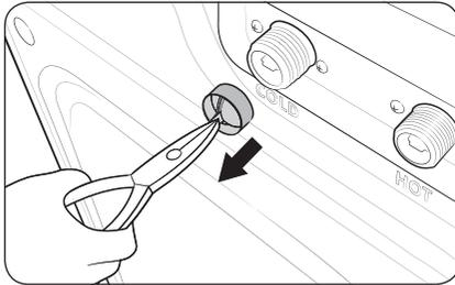
4. Use pliers to pull out the mesh filter from the inlet valves.
