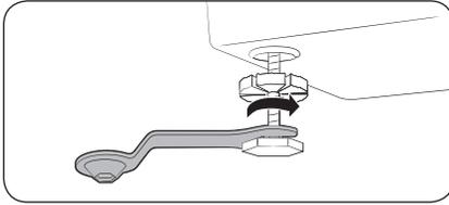
1. Gently slide the washer into position. Excessive force may damage the leveling feet.
