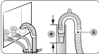
(\*): Min. 6 in. (152 mm), Max. 8 in. (203 mm)
