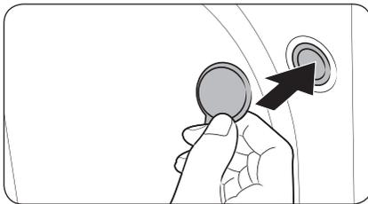
2. Fill the holes with the supplied plastic bolt caps. Keep the shipping bolts for future use.
