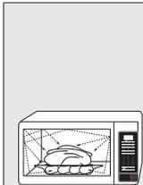
1. The microwaves generated by the magnetron are distributed uniformly as the food rotates on the turntable. The food is thus cooked evenly.
