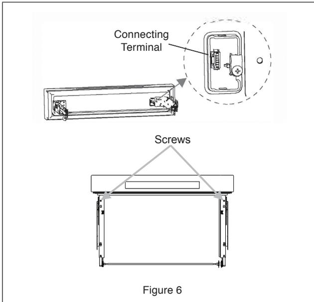
7. Remove the screws on the left and right slideway supports and have one person hold the Flex Drawer door for support.
