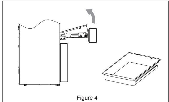
3. Pull the whole tray toward you about 5/8" until the support claws of the slide rails are separated from the tray.
