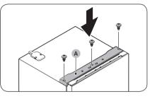
**38**.Insert the **top table (A)**, and then fix it firmly to the refrigerator using the screws (x3).
