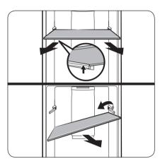
To remove the shelf, hold it with both hands and lift it to release it from the rear hook. Then, tilt it on one side and pull it out.
