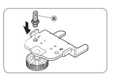
**9.** Insert the **hinge shaft (A)** into the leftmost hole on the bottom hinge plate as shown in the figure, and then tighten it until it is securely in place.
