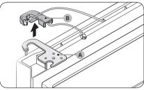
**17.**Remove the **top hinge (A)** with its cover.
