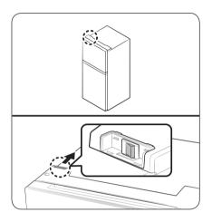
Turning the Auto Ice Maker on or off You can turn the Auto Ice Maker on or off with the switch on the top of the refrigerator.
