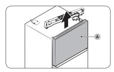
1. Use a Phillips screwdriver to remove the screws on the top table (A). Then, gently pull out the top table (A).
