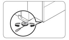
To level the refrigerator, use a flathead screwdriver to turn the leveling leg clockwise or counterclockwise. Turn the leveling leg clockwise to raise, and counterclockwise to lower the height.
