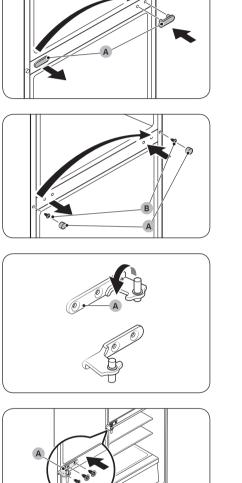
**24.**Use a flat-head screwdriver to remove the **middle-hinge screw cap (A)**, and then reinsert it on the opposite side.
