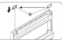
**22.**Remove the **cap spacer (A)**, and then reinsert it on the opposite side.
