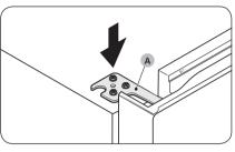
**32.**Insert and fasten the **top hinge (A)** on the opposite side.
