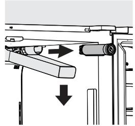
**To Reinstall:** Push the cover up toward the liner, and then push it toward the rear of the cabinet. The filter cover will snap back into place.
