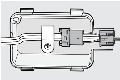
4. Reattach the electrical harness by positioning the cable clips over the black markings on the harness and push the 4 cable clips through the openings in the rail to secure the harness in place.
