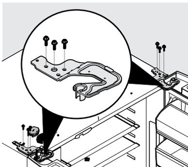
7. In certain circumstances, you may need to remove the lower hinges for clearance purposes. To gain access to the lower hinges, first extend the Custom-Flex Temp Drawer. Unscrew the 3 lower hinge screws and slide the hinge inward.
