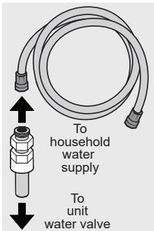
3. Open the locking clips and grab water line coming from the refrigerator. Remove plastic cap from water inlet fitting and discard cap.
