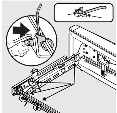
4. Remove the screw and the retaining clip and disconnect the harness
