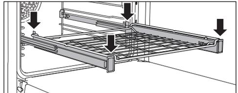
The FlexiClip telescopic runners can support a maximum load of 33 lb (15 kg).
