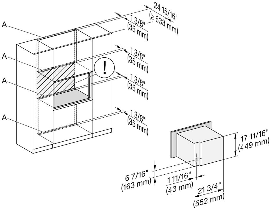
**A** Cutout (min.  $2 \frac{3}{4} \text{ in.}^2$  or  $1800 \text{ mm}^2$ ) for power cord and ventilation
